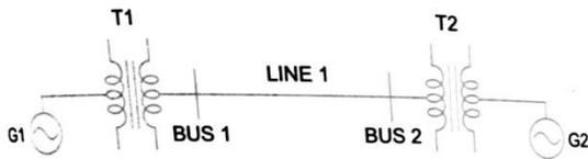
Choose 25 kV as the base voltage at the generator G1, and 200 MVA as the MVA base. The impedance diagram is
